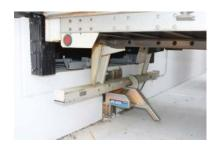
dock while a forklift is operating inside the trailer. Featuring a rotating hook engagement that captures the rear impact guards, the APS 2000 secures the trailer to the dock. Interior and exterior LED green and red lights communicate the status of the dock to the truck driver and forklift operator to ensure safe operation.
